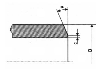
Figure 1 — Tube end bevel
